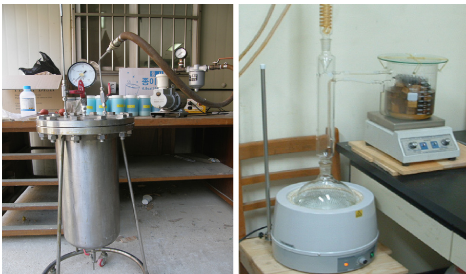
Fig. 1. Images of the laboratory pressure cylinder used for the treatment of preservative formulations (left) and the extraction apparatus used for the hot-water leaching of the wood blocks treated with preservative formulations (right).
